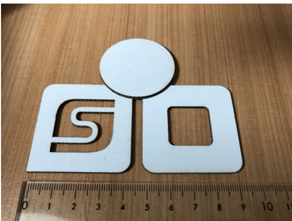
5 - cardboard Solid (white sides) 1.1 mm, F 15 mm/sec, Pwr 255
