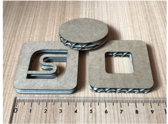
8 - Double corrugated cardboard 6.5 mm, F 10 mm/sec, Pwr 255
